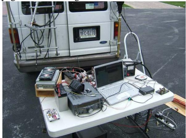
K1DS operating position. You can see the planar reflector of the Wimo antenna in the upper left corner. Here the up angle on the antenna is for EME operation.
