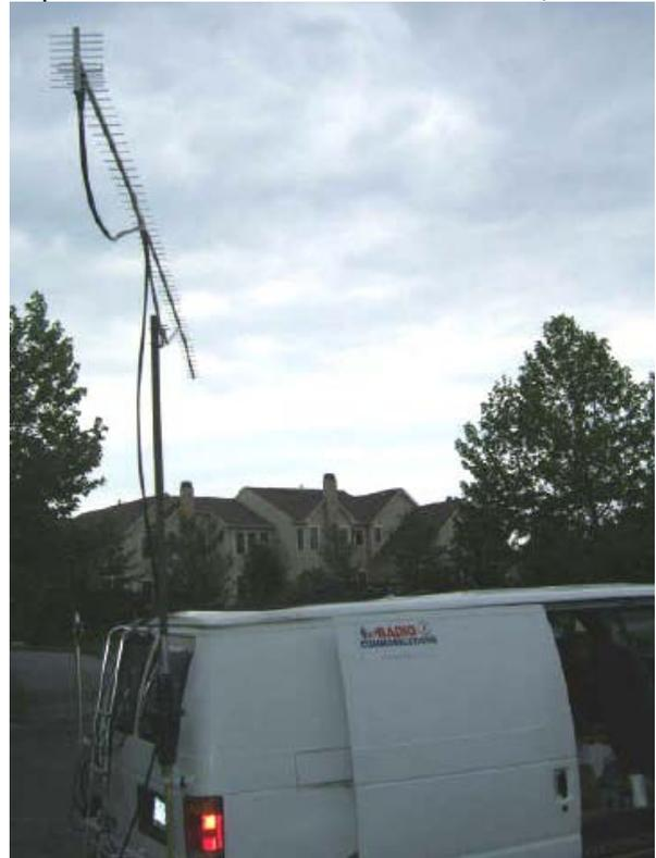
Wimo antenna deployed for terrestrial operation. The antenna is a 67 element SHF yagi with 21.9dBi gain.
