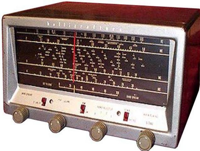
One month later I found a real great deal on a **Hallicrafters S-38E** full four band superheterodyne with a stable BFO for all band AM, SSB, DSB and CW reception. I didn't have to fiddle with the regenerative control. The S-38E had a Beat Frequency Oscillator. I filled three log books with QSO's from 29 states and 12 foreign countries using this rig.
