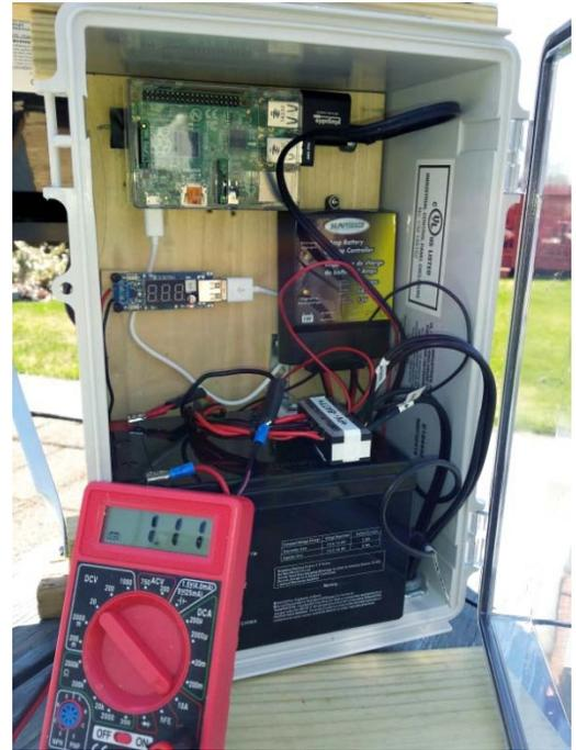
I assembled the whole unit and placed it outside near some wind chimes. The unit worked well during sunny days. During a cloudy stretch, however, I noted a rapid decline in battery voltage and secured another 10 watt panel. Now I am hopeful that the unit has enough charge capability and capacity to keep the unit going through some cloudy days. Kansas will have more sun than Pennsylvania so if I can keep it going here, it should work there.
