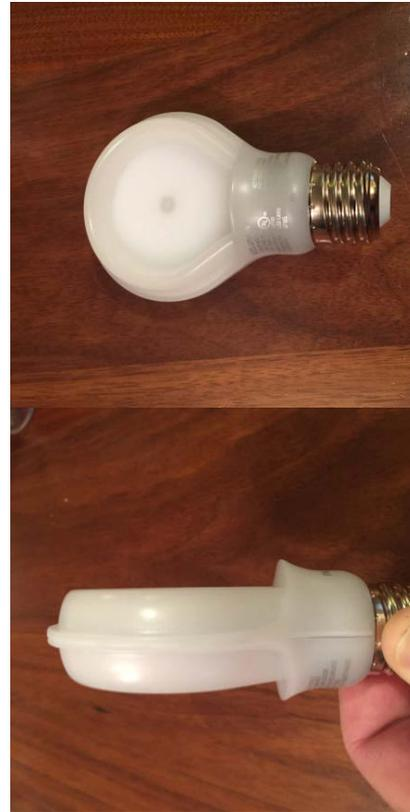
To perform my evaluation, I devised a two pronged approach. First, I set the lamp on my desk in the proximity of both my Yaesu FTDX3000D HF transceiver and my Yaesu FT-8900 VHF transceiver. I listened to the background noise on several bands with the lamp both illuminated and off. I noticed no appreciable difference in the background RF noise received as a result of the LED lamp.
