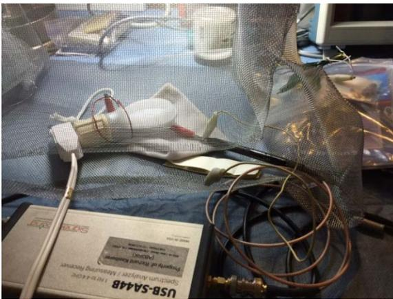
The probe from my SignalHound ® USB-SA44B Spectrum Analyzer was fed into the Faraday Cage with the shield of the probe connected to the grounded cage with a clip lead.
