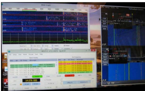
**Screen Photos.** The screen photos show the Flex 6300 on the right and the WSJT-X program on the left. The red lines in the WSJT-X side show a call to me from EA4DKJ in Spain and then the other text lines of the QSO on 14.076 on 8 Sep 15. It is easy to reduce the FLEX screen to half size then activate and use the JTX program to make QSOs. The photos are not as clear as I would like but the dual functions of radio and data program are quite evident.
